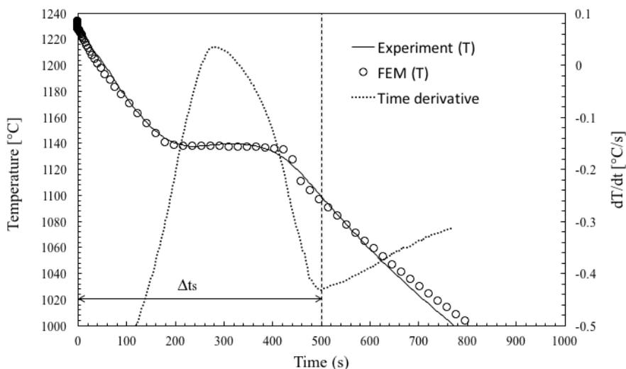
**Fig. 4** Thermal analysis performed on step 1 (**Fig. 1**) and comparison between experimental and numerical temperature history evaluation
