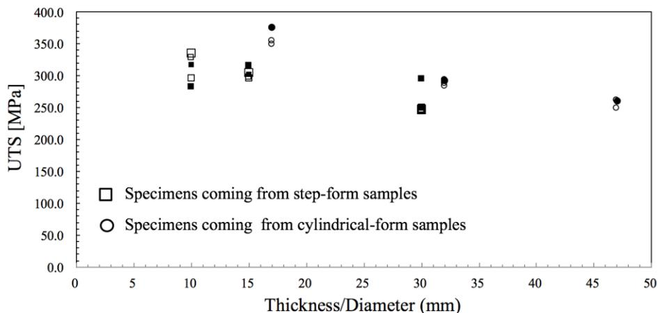
**Fig. 8** UTS of GH 190 GCI as a function of sample thickness/diameter
