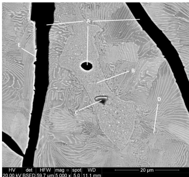
**Fig. 5** SEM micrograph of the analysed alloy showing all its constituents detected: flake graphite (A), steadite (B), manganese sulphides (C), pearlite (D), ferrite (E)
