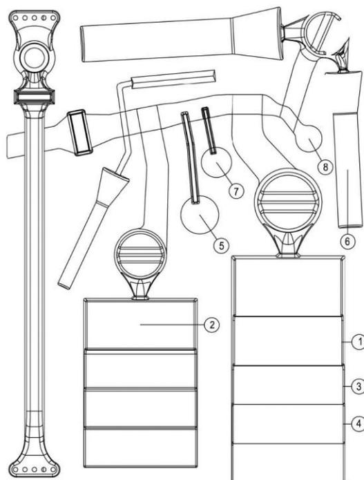
**Fig. 1** Sample geometry used in the experiments. Specimens numbered 5, 7 and 8 are vertical cylinders of diameter 47 mm, 32 mm and 17 mm, respectively. The step-shape geometries are indicated with the numbers 1, 2, 3 and 4 and are characterized by thicknesses of 30 mm, 30 mm, 15 mm and 10 mm, respectively.
