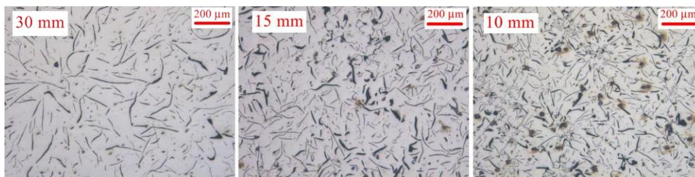
**Fig. 6** Graphite morphology as a function of the step thickness.
