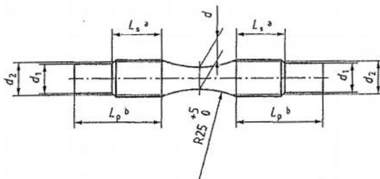
**Fig. 2** Tensile test sample geometry (UNI EN 1561:2011)
